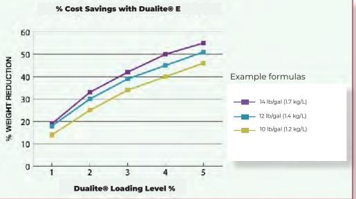
The chart demonstrates the percent weight reduction for formulas with initial specific gravities of 10, 12, and 14 pounds/gallon (1.2, 1.4, and 1.7 kg/liter) at different loading levels of Dualite® E065-135D.
